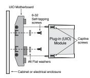
**SIGA-CC2A:** mount to North American 2-1/2 inch (64 mm) deep two-gang boxes and 1-1/2 inch (38 mm) deep 4-inch square boxes with two-gang covers and SIGA-MP mounting plates. The terminals are suited for #12 to #18 AWG (2.5 mm<sup>2</sup> to 0.75 mm<sup>2</sup>) wire size.
